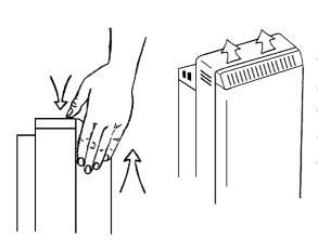
Remove the front panel/grille assembly by removing the two screws along its bottom edge. With hands positioned on either side of the panel, lift upwards to unhook the top edge whilst pressing down on the top panel with your thumbs. The panel can now be lifted clear and set to one side.
