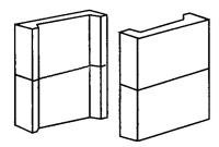
Note the way the bricks are positioned in the heater. Otherwise, they will not fit.
