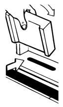
Put in place the rear rank of bricks, pushing them well back against the rear insulation. Replace the element, making sure that the connection is tight.
