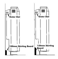
A clear space of at least 3" (75mm) must be left at either side of the heater, and any projections or shelves must be at least 10" (250mm) above the heater casing. Curtains must not be draped around or in contact with the casing. A shelf unit is separately available for fitting above heaters.
