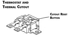
However if the cutout has operated, determine the cause of the cutout operating. If the heater has not obviously or inadvertantly been misused - e.g. covered - it will be necessary to have the appliance fully checked by a **Creda Service Agent**
