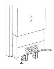
There are two fixing slots at each end of heater, allowing different stand-offs for different thicknesses of skirting board. Do not fully tighten these screws until the bricks are loaded into the heater as some settling of the heater may occur. NOTE: NEVER REMOVE THESE SCREWS WITHOUT FIRST UNLOADING THE HEATER.
